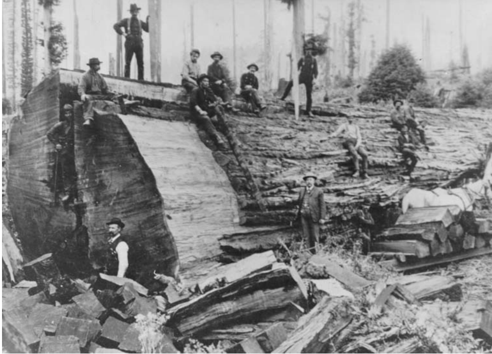
Figure 203. Huge trees were sometimes “bucked up” (cut into sections) with whip saws to make railroad ties, grape stakes, shingles, or other split goods. (Photo courtesy Humboldt Redwood Company, formerly Pacific Lumber Company.)
