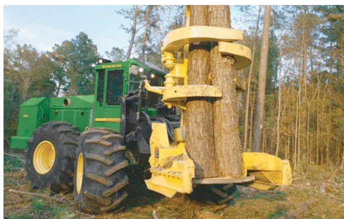
Figure 210. Wheeled feller-buncher. The circular saw blade is at the bottom of the group of trees. (Photo courtesy John Deere Corp.)
