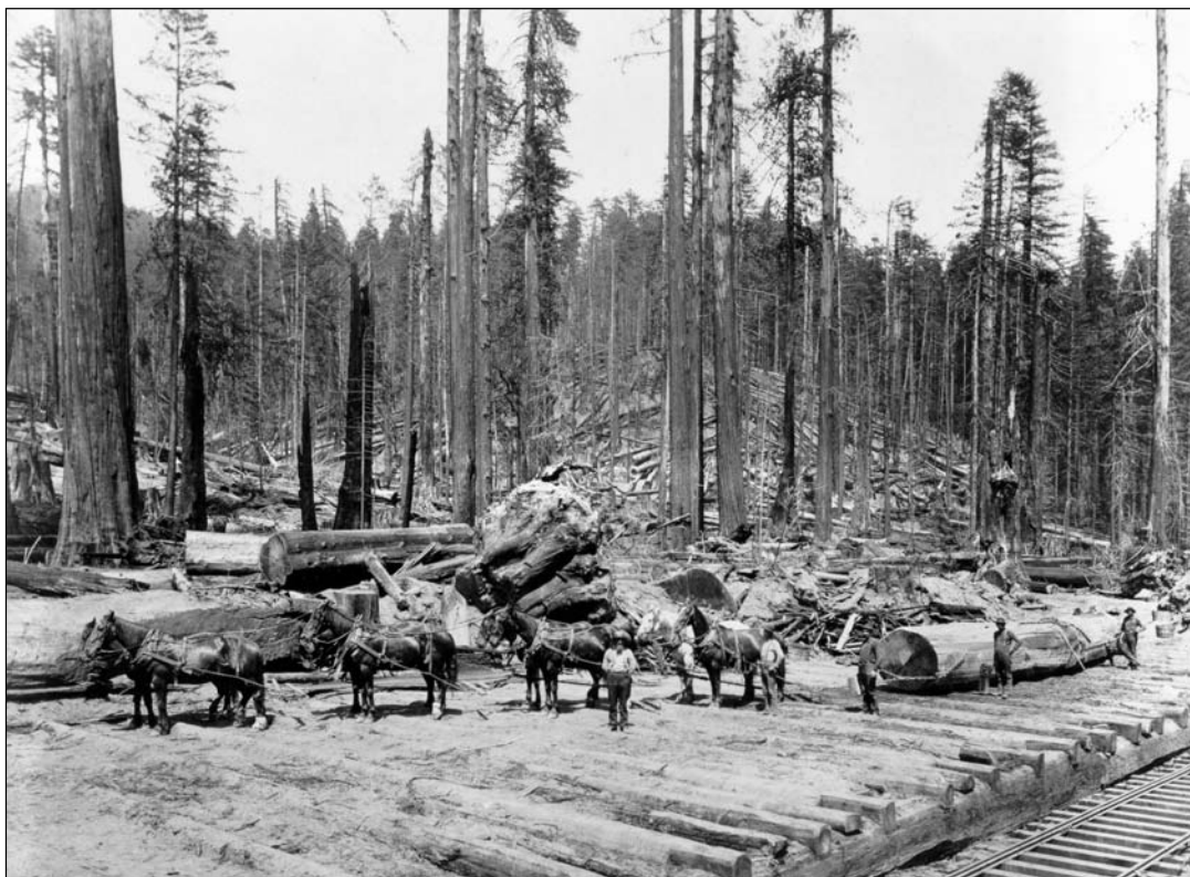
Figure 197. Teams of mules or horses were used to drag logs to the rail landing, or to a river. Skid trails of logs were made to keep the logs from digging into the ground. Many trees were often left standing because only the best trees were cut. (Photo courtesy of Humboldt Redwood Company, formerly Pacific Lumber Company.)
