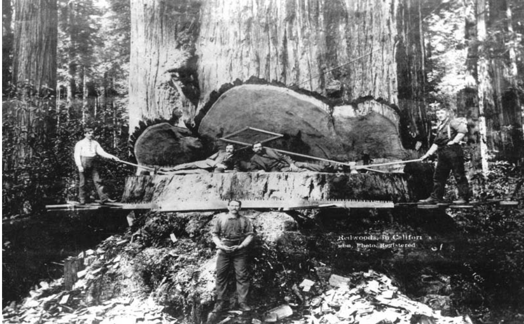
Figure 195. Logging with axes was hard, dangerous, time-consuming work. To fell the large trees, special axes with longer handles were made. The introduction of the whipsaw made the felling of the giants easier and faster. Note the springboards and the waste chips around the base of the tree. (Photo courtesy Clarke Museum.)
