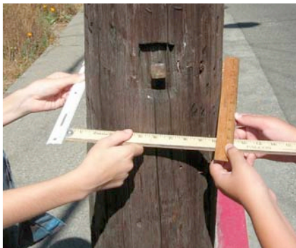
Figure 187. Measuring a pole's diameter: Make a "caliper" using a yard stick and two rulers held perpendicular to it (parallel to each other).
