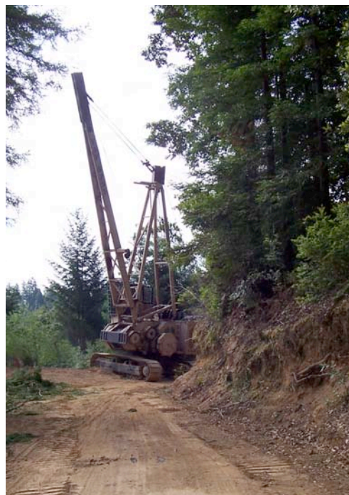
Figure 212. The use of a cable yarder operating from high on the hillside or on the ridge enables logs to be pulled uphill rather than dragged through stream beds. Compare this picture with Figures 200 and 205. (Photo courtesy of Mendocino Redwood Company.)
