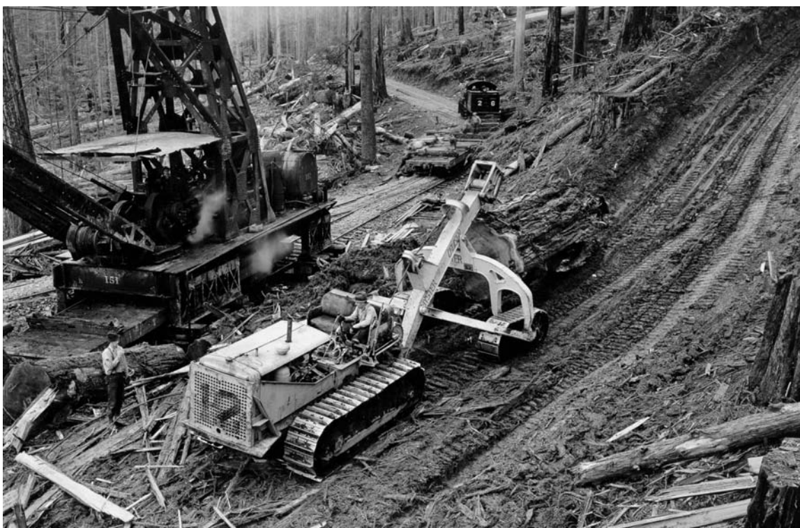
Figure 205. Tractors with “caterpillar” treads or “tracks” allowed dragging of the huge logs from the forest, but caused much soil disturbance, resulting in erosion of soil into the streams. (Photo courtesy of Humboldt Redwood Company, formerly Pacific Lumber Company.)
