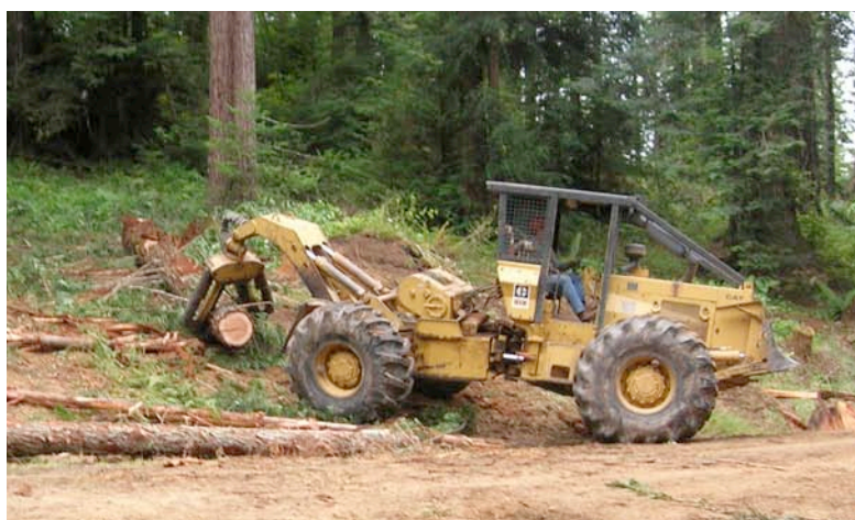
Figure 211. Skidder bringing a log to a landing, where it will be loaded onto a truck.
